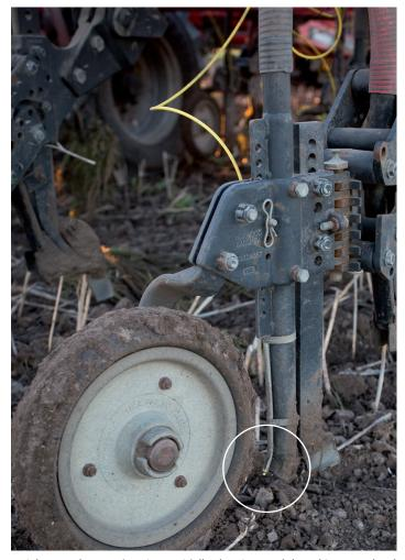
stainless steel protective pipes. Initially, the pipes and the tubing were level with one another, but they found this set-up was prone to blockages, so adjusted the tubes to sit 3mm to 5mm below the pipes. "The tubes now flicker, which prevents any blockages. Peter didn't get a blockage at all last year," said Craig.
