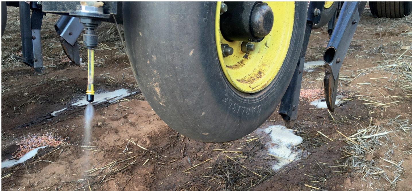
Above: Shows the split terminal configuration, the nozzle on the left is behind the press wheel & applies the surfactant. The other liquid line is on the front (right) seed tine. Below: Control strip with no wetter surfactant & trace elements on non wetting soil stands out.
