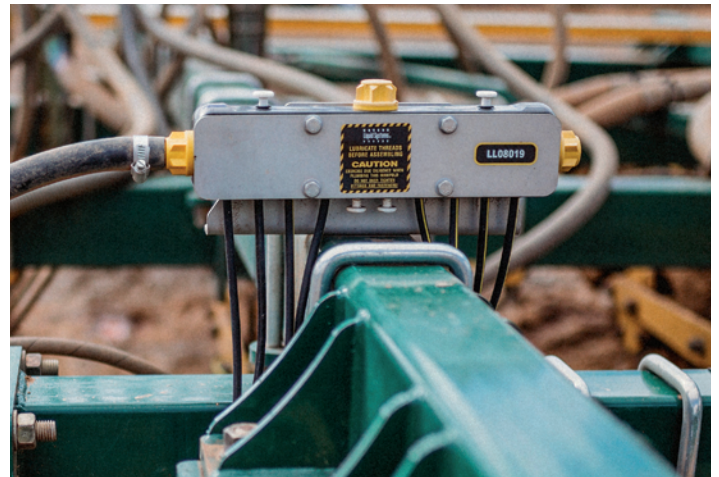
Left: A120 (126L/min) Pump & Control Module has been mounted on the bar. Right: Six “Stacker” manifolds are mounted on the bar, with 50 terminal outlets using friction tube. Below: L-R, Dustin Sparrow, Lyndon Kloeden and Paul Sargent.
