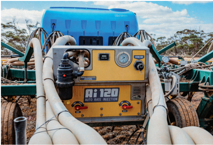
Left: A120 (126L/min) Pump & Control Module has been mounted on the bar. Right: Six “Stacker” manifolds are mounted on the bar, with 50 terminal outlets using friction tube. Below: L-R, Dustin Sparrow, Lyndon Kloeden and Paul Sargent.
