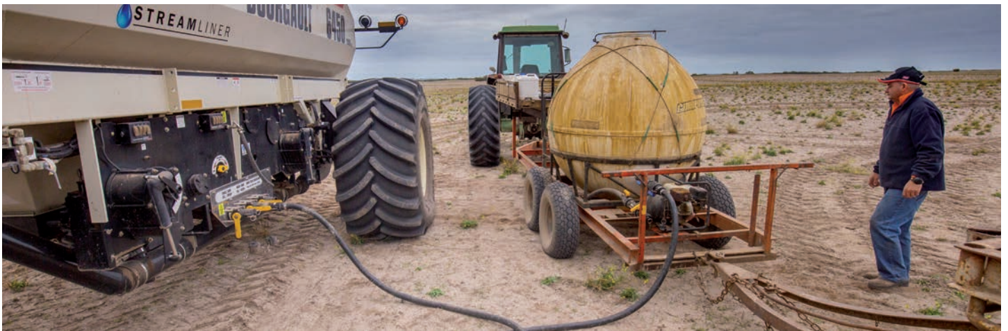
Opposite page: A120 (126L/min) Pump & Control Module is neatly mounted on the back of the Bourgault 6450AU Cart. Above: Michael transferring liquid from his converted boom sprayer, 2000L tank to his air cart. Below left: Liquid stream from friction tube assembly. Below right: Michael Shepley
