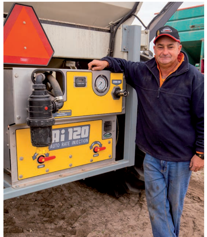
Opposite page: A120 (126L/min) Pump & Control Module is neatly mounted on the back of the Bourgault 6450AU Cart. Above: Michael transferring liquid from his converted boom sprayer, 2000L tank to his air cart. Below left: Liquid stream from friction tube assembly. Below right: Michael Shepley
