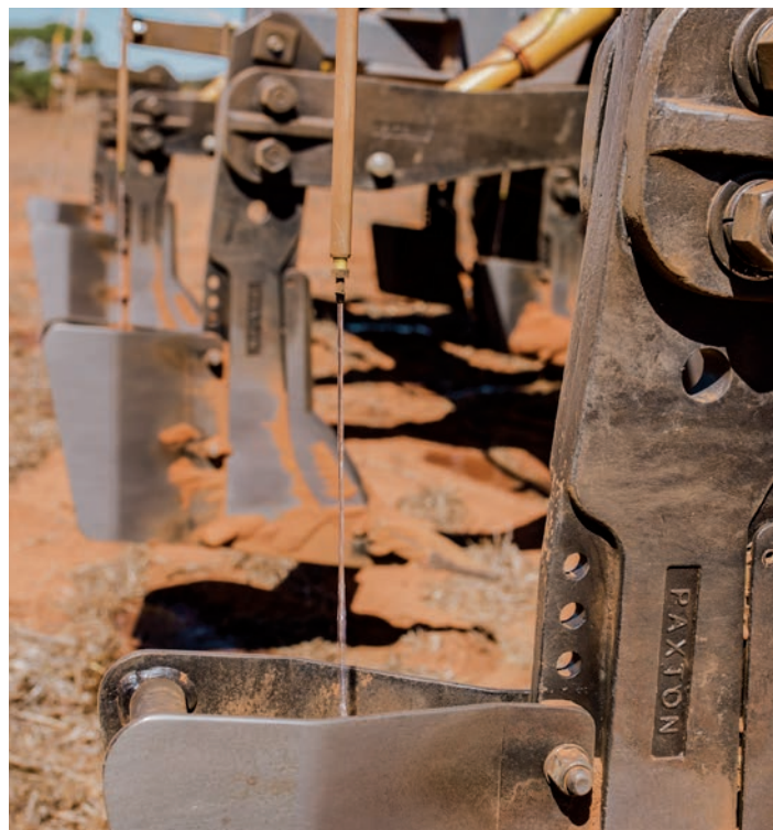
Font page image: Tristan Baldock in front of the rig. Above left: In cab dashboard, including the Famscan Jackal Liquid Controller. Above right: Close up of the liquid stream. Below: back view of the Paxton Plow with liquid terminal assemblies.
