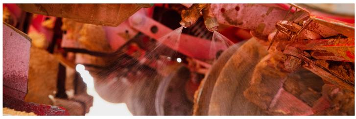
**Opposite page:** Peter Corcoran in front of his Liquid Systems Spiker Module **Above:** The Spiker module is used to spray in-furrow a mix of fungicide, insecticide and bio-stimulant into the potato root zone during planting. **Below:** Corcoran planting potatoes using the Spiker Module, mounted to the John Deere Tractor pulling the six-row Grimme potato planter.
