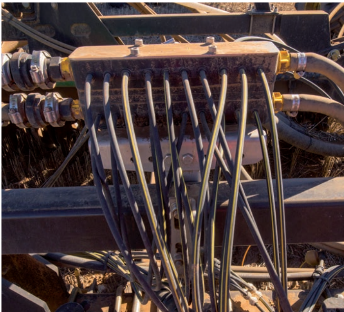
Front page: Nathan Clifford (left) & Wick Daymon (right) in front of their Spiker & G22 Modules. Above left: One of five dual Stacker Manifolds, allowing 98 outlets in total. Above right: Close up of liquid stream & terminal assemblies mounted to the K-Hart disc seeder with Gent Openers. Below: Warbuto Farms complete seeding rig in action.
