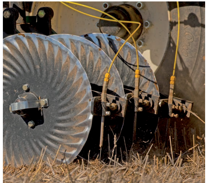
Front page: Nathan Clifford (left) & Wick Daymon (right) in front of their Spiker & G22 Modules. Above left: One of five dual Stacker Manifolds, allowing 98 outlets in total. Above right: Close up of liquid stream & terminal assemblies mounted to the K-Hart disc seeder with Gent Openers. Below: Warbuto Farms complete seeding rig in action.
