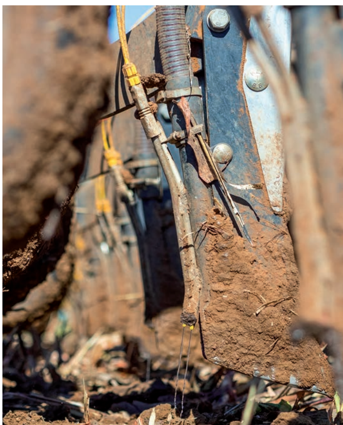
Front page: The two liquid rigs in the field. Top: Phill Coggan in front of his two LQS120 Modules mounted on one of the liquid carts. Left: Dual outlets, independent liquid application mounted on the Horsch Tynes
