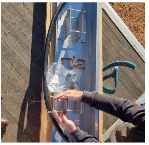
• Loosen the clamp to fascia bolts to allow the clamps to expand over the air cart frame.
