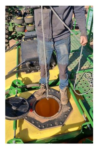
• Slide the tank fitting and gasket down the rope and through the hole in tank.
