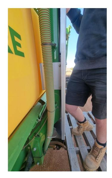
• Push the assembly firmly against the frame, reinsert the removed through bolts and tighten all 4 bolts of each clamp mount until firm.
