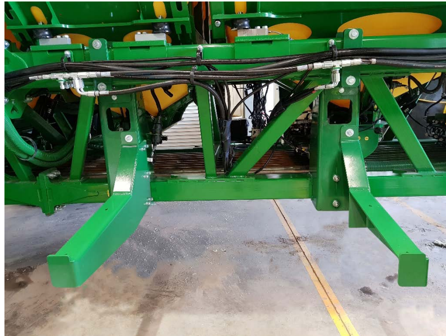
Support Frames mounted onto TBH Chassis
