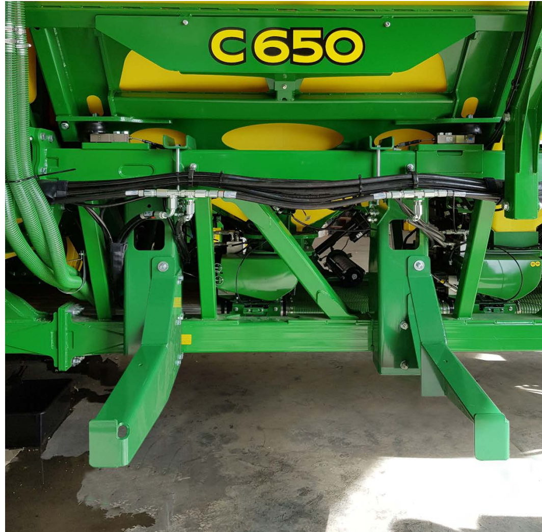
Support Frames mounted onto TBT Chassis
