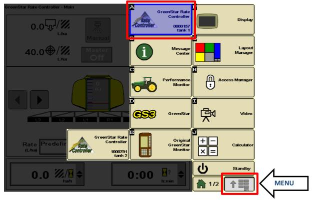
Select **Setup** button to enter GRC setup. Select **Implement** tab. Select **Liquid Fert. Tool** as implement type. Select **New** to create a new Implement name or select an existing name.
