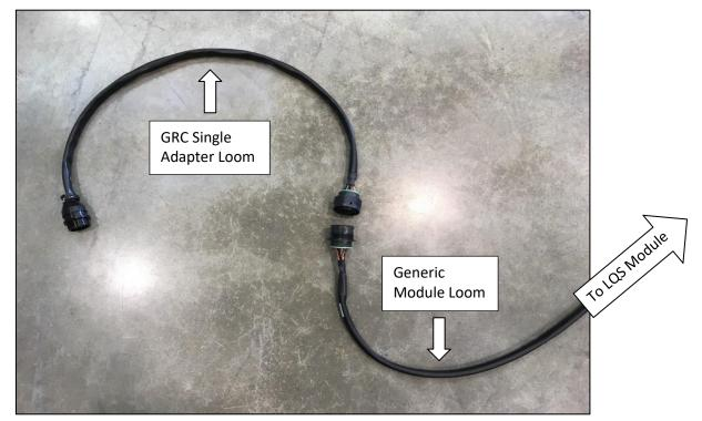
4. Connect GRC Single Adapter Loom to GRC Main Harness.
