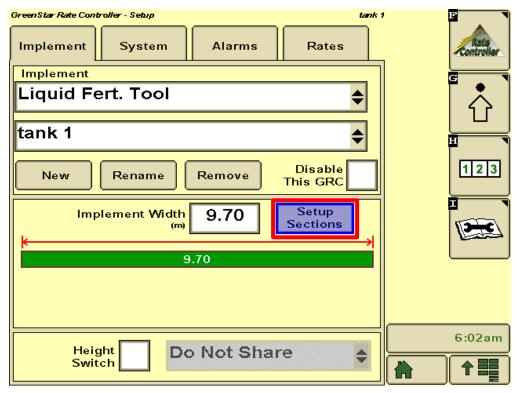
Enter 1 for single section setup and press **Next Page** button (right arrow).
