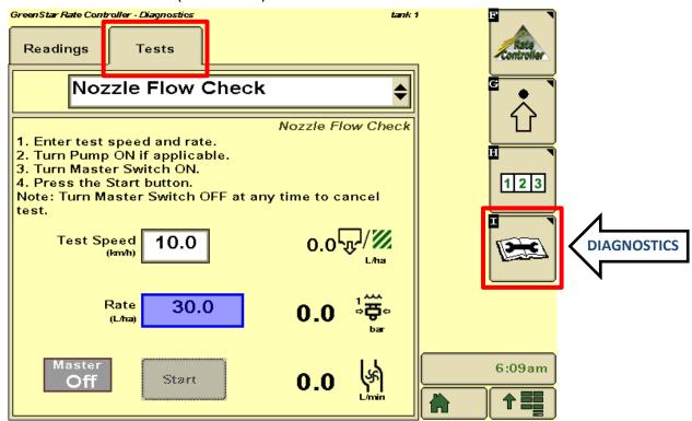
If rate control is erratic, go to **System Setup** screen and adjust **Control Valve Calibration** values to optimise performance. Increase first 2 digits for faster response, decrease for smoother control. Refer to GreenStar Rate Controller Operator's Manual for more information.
