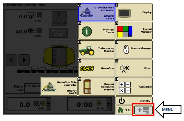
Select **Setup** button to enter GRC setup. Select **Implement** tab. Select **Liquid Fert. Tool** as implement type. Select **New** to create a new Implement name or select an existing name.
