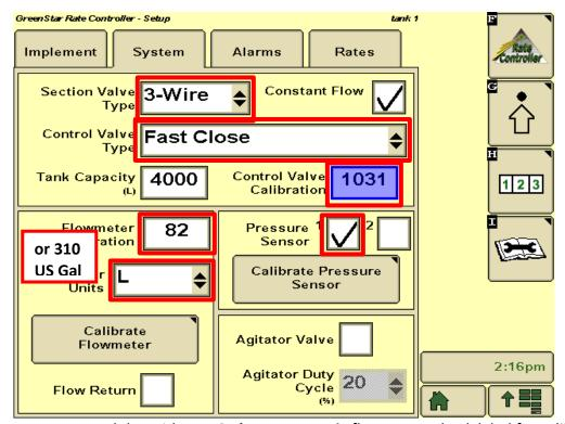
Note: For modules with ARAG Electromagnetic flowmeter, check label for calibration number.
