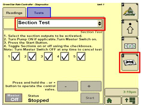
2. Turn the Master switch on and press **Start** button to start the test. Ensure all sections are open.
