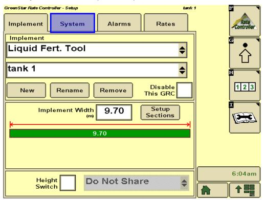
Select **3-Wire** for Section Valve Type from drop down menu.
