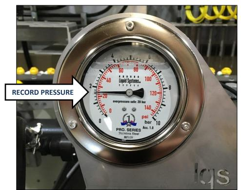
Ideally the pressure should be similar to pressure at typical operating rate and speed. Adjust pressure with the onscreen – and + buttons on screen if the pressure is too high or low.
