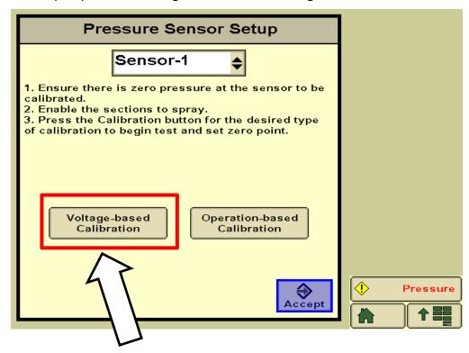
Enter Pressure Sensor Calibration factor 5mV/kPa : 500mV/bar : 34.5mV/psi Press **Accept**.
