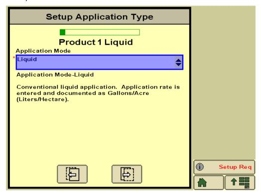
Setup single section as below. Press **Next Page** button (right arrow). If required, press **Previous Page** button (left arrow) to go back and re-enter data.
