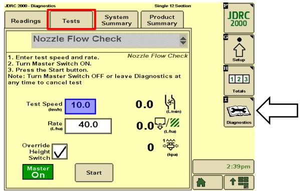
If rate control is erratic or slow, go to **Control Valve Setup** screen and reduce **Valve Response Rate**
