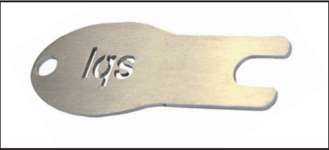
(Use the Compression Tool to depress the Locking Collets on the STACKER Manifold quick release insert cartridges when inserting or extracting the 8.0mm PE tubing.)
